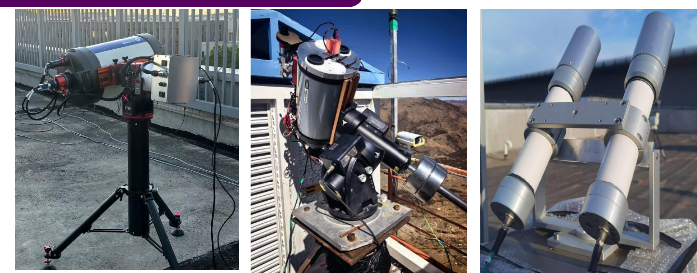
Fig. 6. Representative ground-based optical-turbulence monitoring instruments used in the joint observation campaigns.
